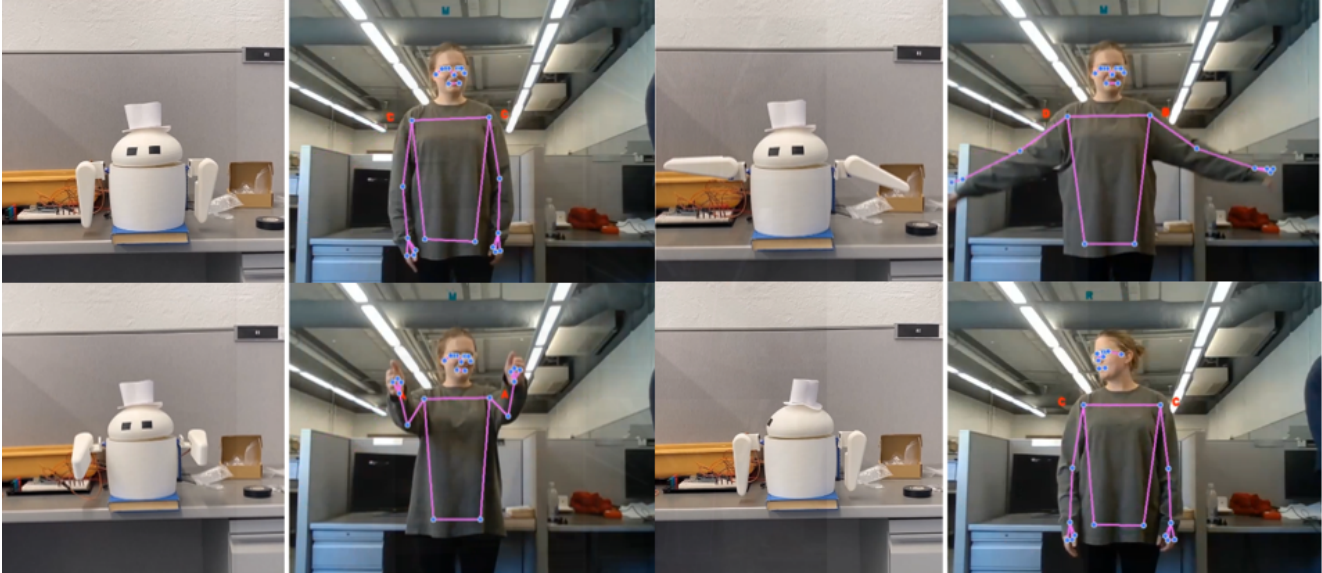
Figure 6. Demonstration of human pose estimation for use in robotic teleoperation
